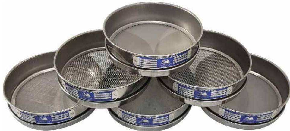
Ø200 x 50 mm Woven Wire Mesh Sieves
