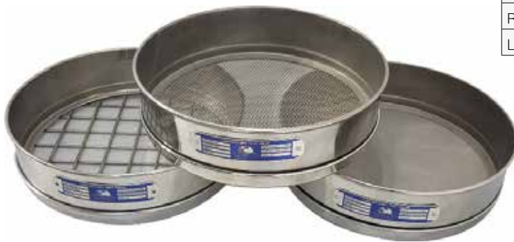
Ø300 x 50 mm Woven Wire Mesh Sieves
